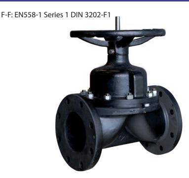
KDV's range of bi directional Weir Type diaphragm valves offer exceptional durability and reliability. The clean design completely isolates line media from the mechanical components of the valve. Bubble tight shutoff (Class VI) and in-line serviceability (top entry) maximise plant efficiency and productivity.
